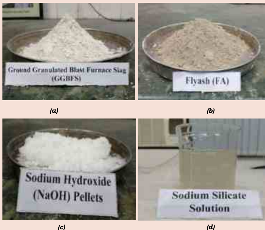
Figure: Cementitious binder and alkali activators used for development of geopolymer concrete mix: (a) Ground granulated blast furnace slag (b) Fly ash (c) Sodium Hydroxide (d) Sodium Silicate solution
